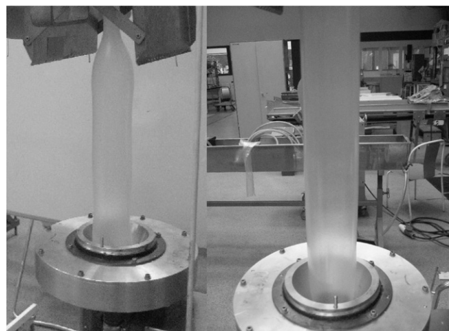
Fig. 3. Film blowing of HONPS 22, at the start of blowing (left) and after some time when the bubble is stable (right).
